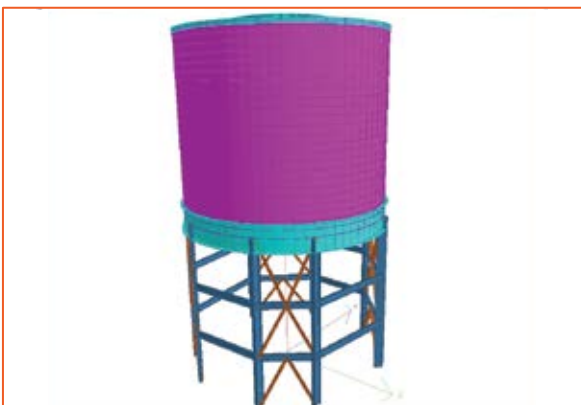
1973 m 3 Silo for Cement Industry in India
