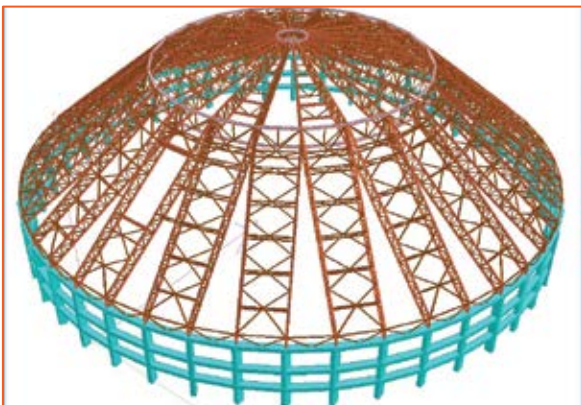
115m Diameter Dome Structure for Lime Stone Storage in India
